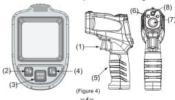
(1) Measurement switch (trigger).
